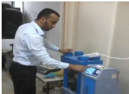
Figure 3.5 Compressive strength test at the lab
