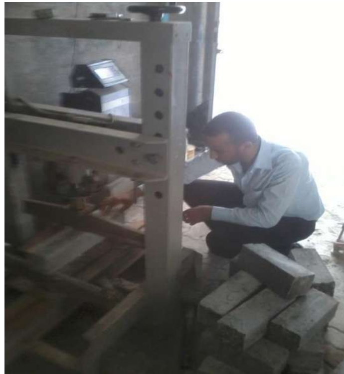
Figure 3.6 flexure tests at the lab
